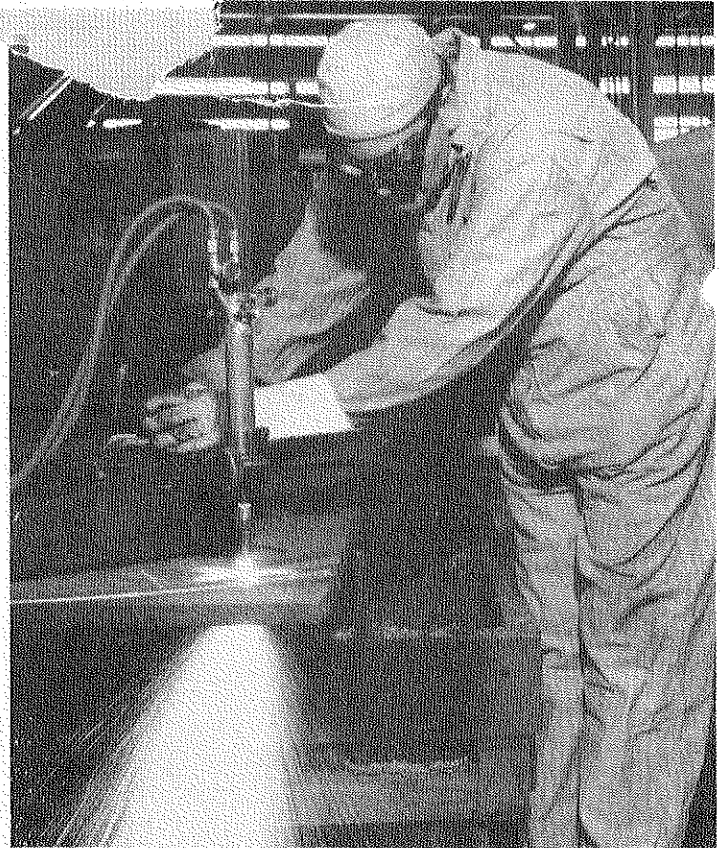
WILLIAM E. BROWNING is pictured using an automatic Oxweld cutting machine. At the time the photograph was taken he was machine cutting a part for the Machine Shop. Welding is one of the many types of occupations required to operate a gaseous diffusion plant.
