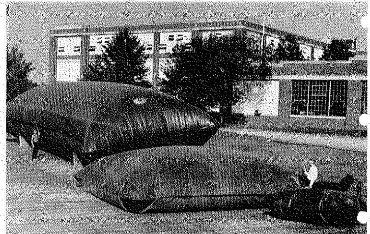
GIANT ECONOMY SIZE — Goodyear inspectors use walkie-talkies to contact each other as they scrutinize three pillow tanks. The rubber and fabric tanks, in sizes up to 100,000 gallons, are produced for a variety of liquid storage and handling assignments. These three tanks, filled with air for test purposes, have 900-, 5,000- and 50,000-gallon capacities. They are made at the Rockmart, Ga., plant.
