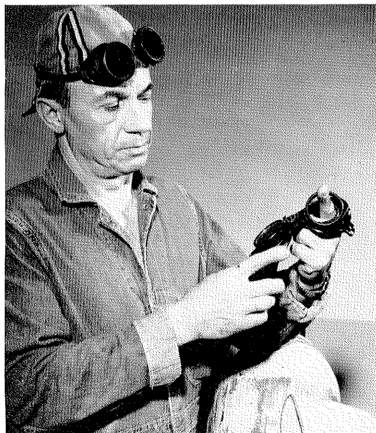
GOGGLES SAVE WELDER'S SIGHT. Ralph DeAmicis (D-732) escaped serious eye injury by wearing protective welding goggles. A bracket which he was cutting snapped out of alignment striking his goggles, shattering the cover lens and cracking the inner protective lens. Ralph was knocked down yet received eye protection from his safety goggles. Ralph's wise use of safety equipment won him membership in the Wise Owl Club of America sponsored by the National Society for the Prevention of Blindness.
