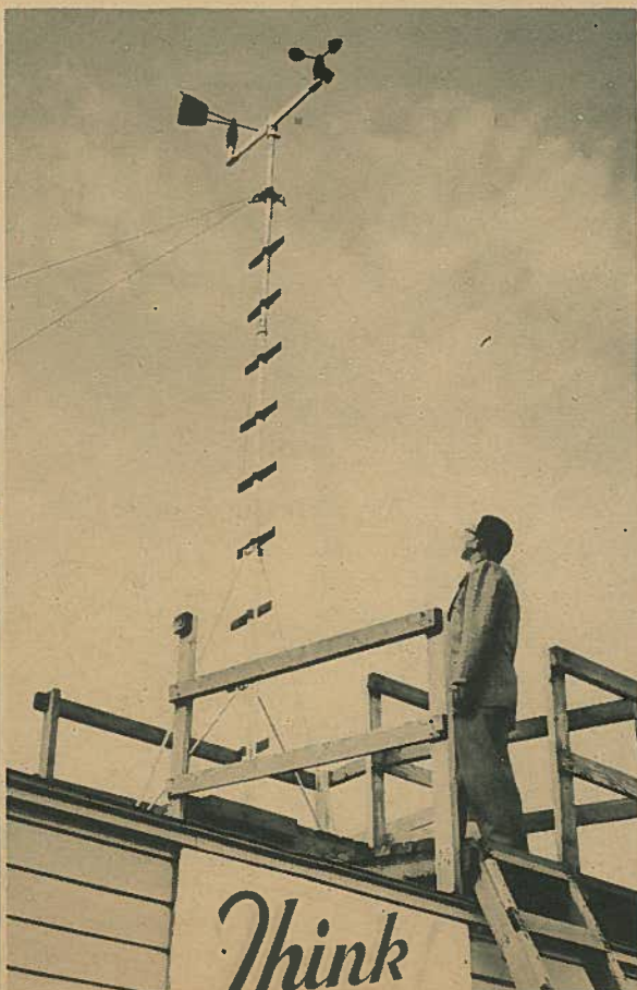
Checking recording equipment at the project weather laboratory is Meteorologist Donald H. Pack of the AEC Portsmouth Area staff. In the left-hand photo Pack is shown taking a reading from the anemograph, an instrument which measures velocity and direction of the wind. At right Pack observes antenna apparatus atop the laboratory north of the Administration Building.
