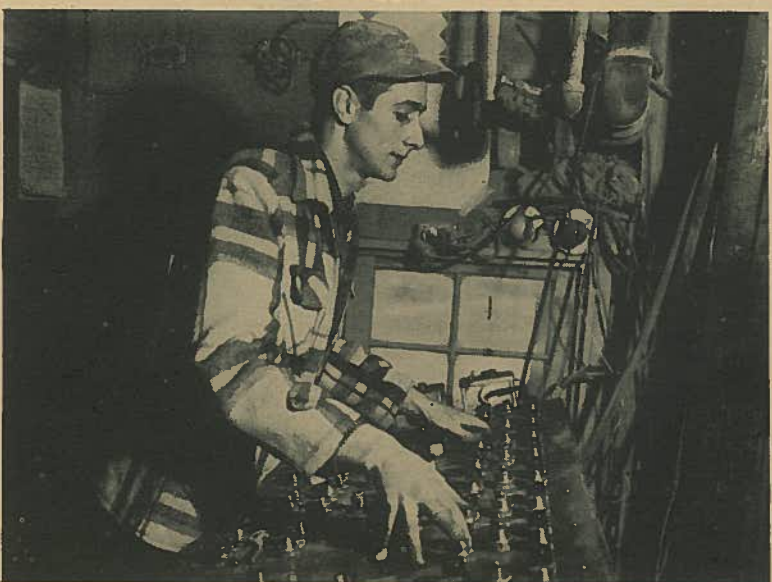
Watching one of the batch plant's four large mixers empty a load of concrete into the bin to await removal by truck is Kolinski's plant operator Rex Whitted. From the large electric board shown above Whitted controls the mixing of hundreds of yards of concrete each day.
