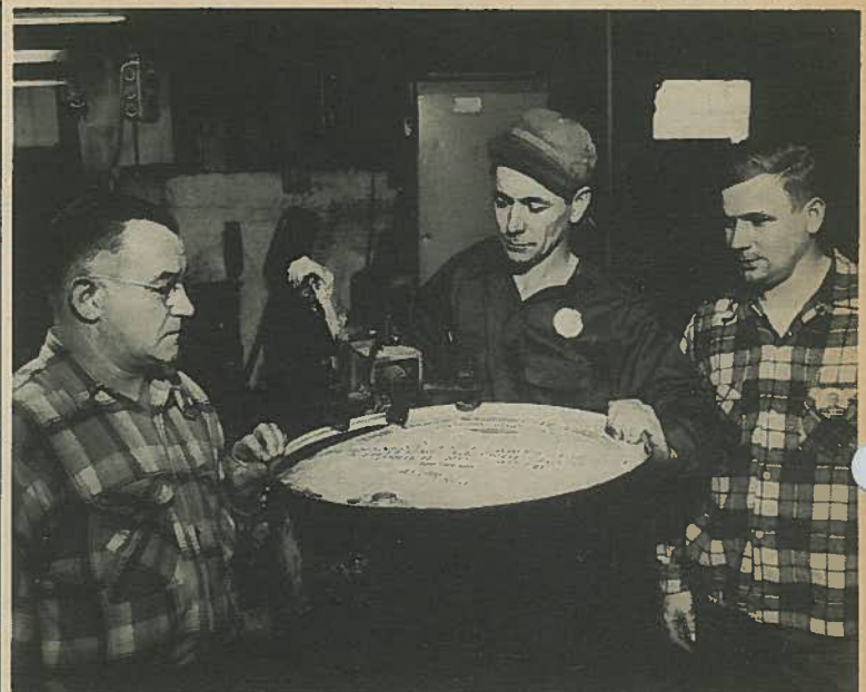
Shown above are the men responsible for the creation of a safe and efficient barrel opener being used at the Portsmouth area project. Pictured operating the device is its inventor, Marvin Schaa. Watching the roller neatly cut through the barrel top is (left) Roy Trein, and (right) William Diefenbach.
