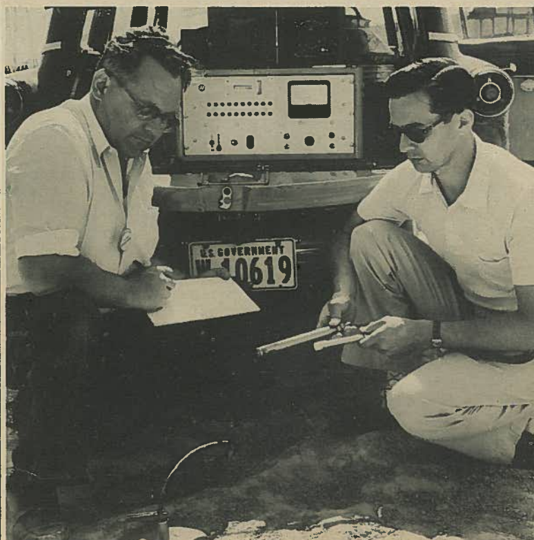
The practical application of radioactive substances is being demonstrated in the above photograph of representatives of the Corps of Engineers in Cincinnati. Harold Brown, left, and engineer-scientist Paul Carlton recently visited the plant site to determine the density and moisture content of the soil at various locations on the job.
